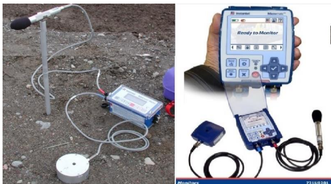
Figure 5. Instantel Minimate Blaster model and Micromate model vibration and air shock measurement devices
