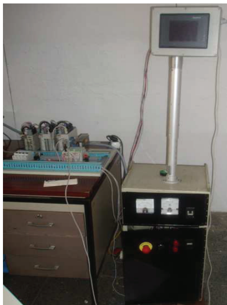
Figure 7. The designed power supply unit training set
